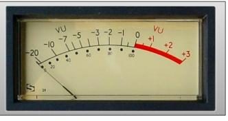
an active rectifier circuit with level adjustment. The attack and release time is 300 ms. The lead can be adjusted to any desired value.
